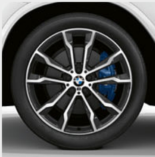
□ 20" M light alloy wheels Double-spoke style 699 M in Bicolour Orbit Grey, gloss-lathed 1,3 , with mixed tyres and run-flat properties, front 8J x 20 with 245/45 R20 tyres, rear 9.5J x 20 with 275/40 R20 tyres.
